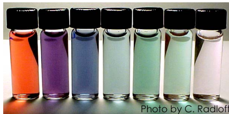
Au and thin gold layers on silica.
